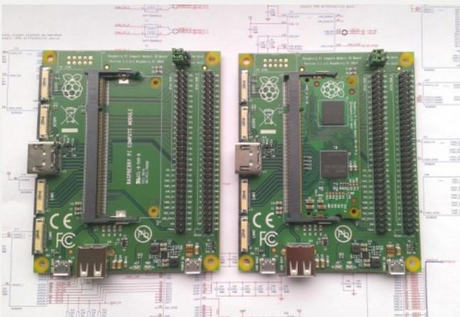
Empty IO Board on the left: Compute Module snapped into place on the right.
