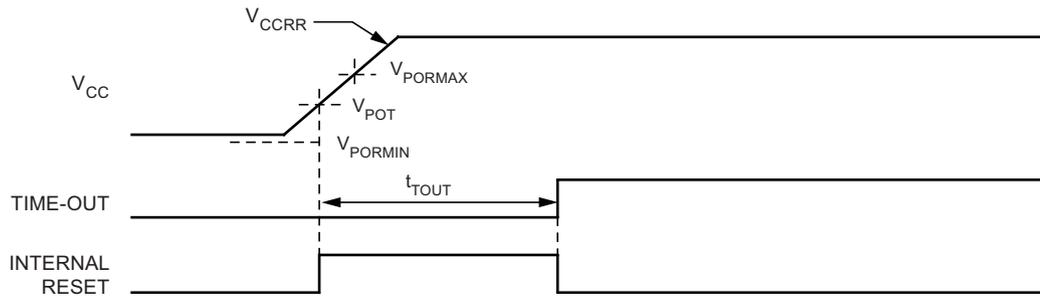
**Figure 5-18. MCU Start-up,  $\overline{\text{RESET}}$  Extended Externally**
