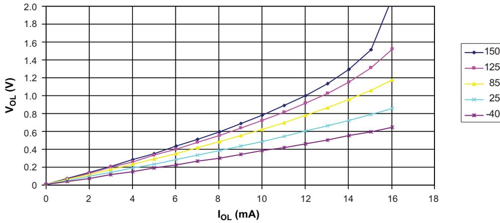
**Figure 5-129. I/O Pin Output Voltage versus Sink Current (V<sub>CC</sub> = 5V)**
