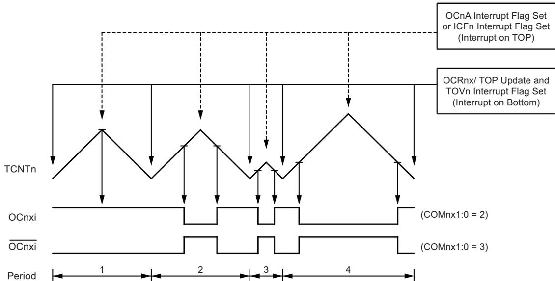
The Timer/Counter Overflow Flag (TOV1) is set at the same timer clock cycle as the OCR1A/B Registers are updated with the double buffer value (at BOTTOM). When either OCR1A or ICR1 is used for defining the TOP value, the OC1A or ICF1 flag set when TCNT1 has reached TOP. The interrupt flags can then be used to generate an interrupt each time the counter reaches the TOP or BOTTOM value.
