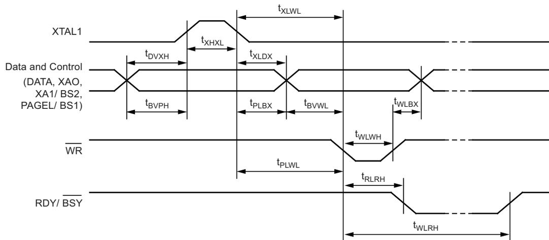
**Figure 5-110. Parallel Programming Timing, Loading Sequence with Timing Requirements<sup>(1)</sup>**
