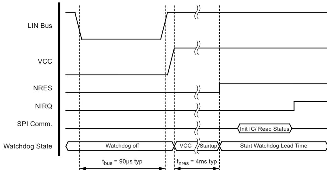
With the initialization of the configuration register by the microcontroller, the status word of the LIN-SBC is transmitted back, including the wake-up source. In other words, the two status bits "IRQS1" and "IRQS0" both read back as '1'. For more information see Section 4.7 "Serial Programming Interface (SPI)" on page 19.
