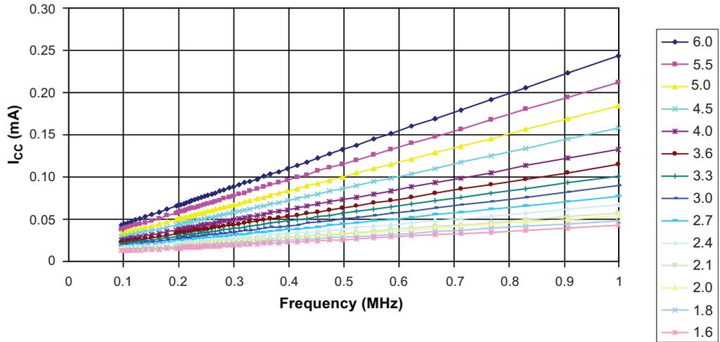
**Figure 5-135. Reset Supply Current versus Vcc, Frequencies  $\geq 1$  MHz
