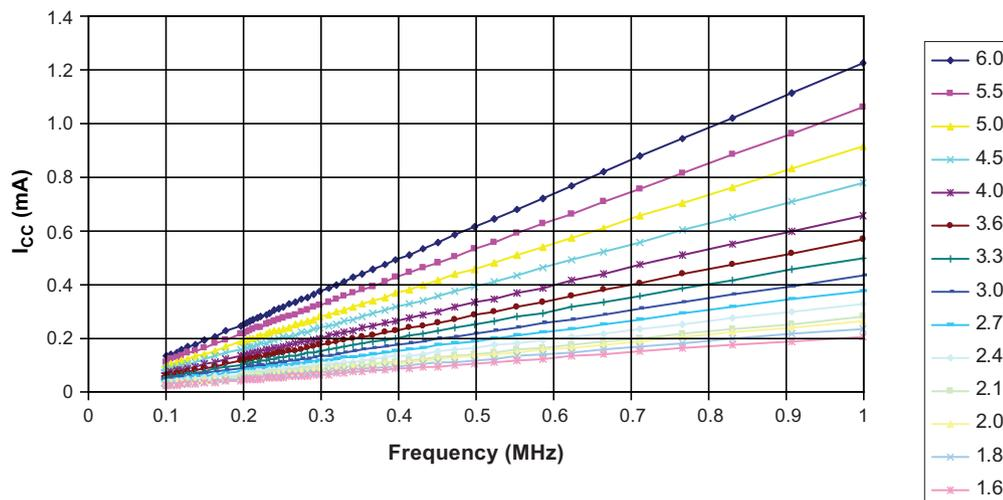
Figure 5-116. Active Supply Current versus Frequency ( $\geq 1$ MHz)
