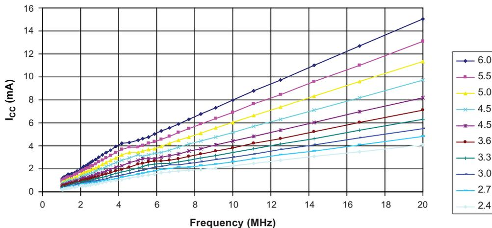
Figure 5-117. Active Supply Current versus  $V_{CC}$  (Internal RC Oscillator, 8MHz)
