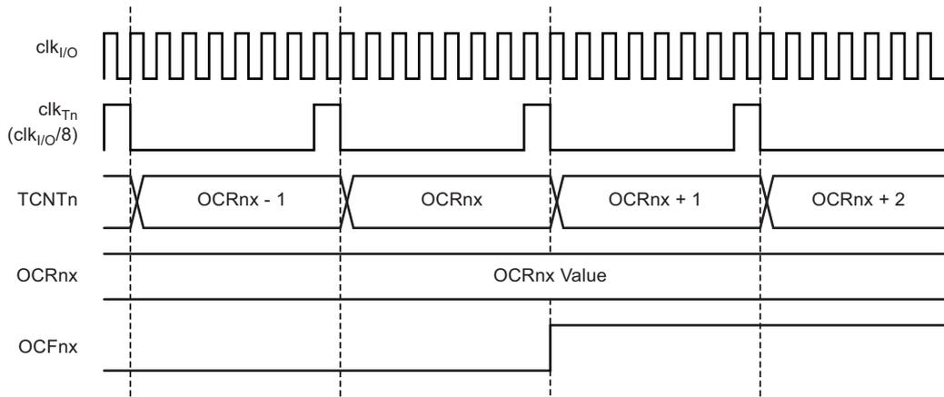
Figure 5-40 shows the setting of OCF0A and the clearing of  $TCNT0$  in CTC mode.
