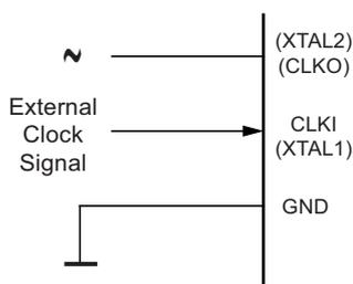
When this clock source is selected, start-up times are determined by the SUT Fuses or CSUT field as shown in [Table 5-12](#). This external clock can be used by the asynchronous timer if the high or low frequency Crystal Oscillator is not running ([See "Enable/Disable Clock Source" on page 69](#)). The asynchronous timer is then able to enable this input.
