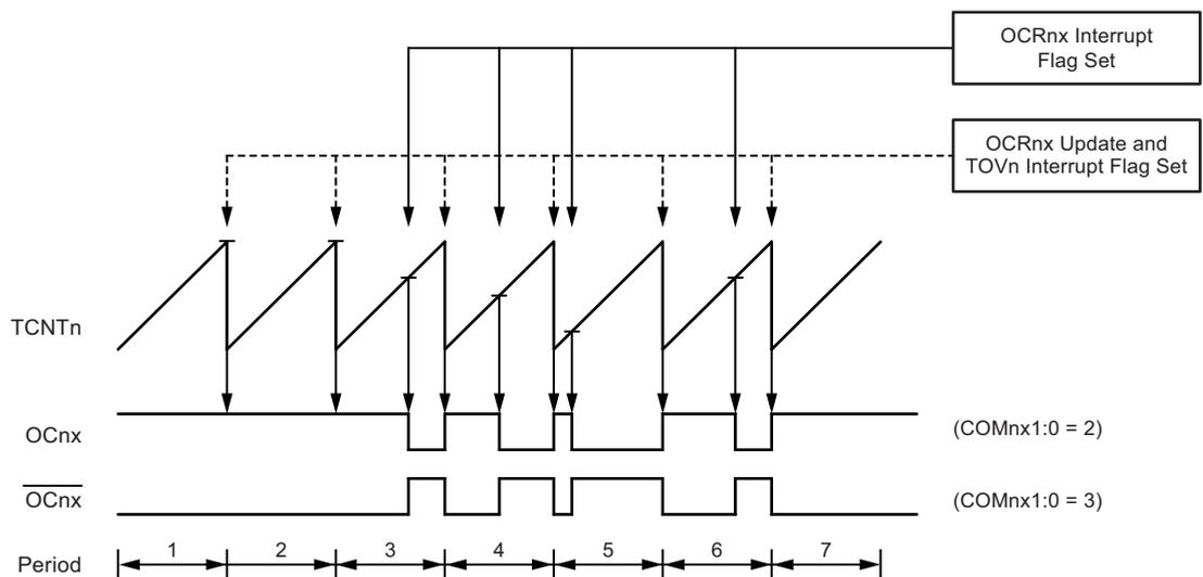
The Timer/Counter Overflow Flag (TOV0) is set each time the counter reaches MAX. If the interrupt is enabled, the interrupt handler routine can be used for updating the compare value.
