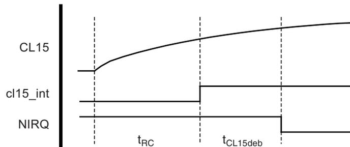
In the diagram above, the voltage at the CL15 pin is shown. Due to the R/C filter, the voltage does not immediately increase but instead slowly over time. As soon as the voltage exceeds approximately 3V, the internal debouncing time  $t_{CL15deb}$  starts. After this elapses, a wake-up is indicated by a falling edge on the NIRQ pin.
