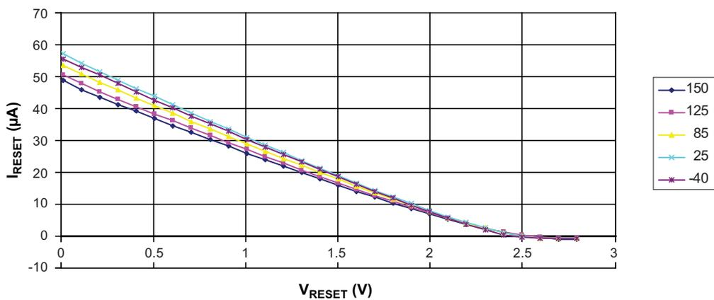
**Figure 5-127. Reset Pull-up Resistor Current versus Reset Pin Voltage (V<sub>CC</sub> = 5V)**
