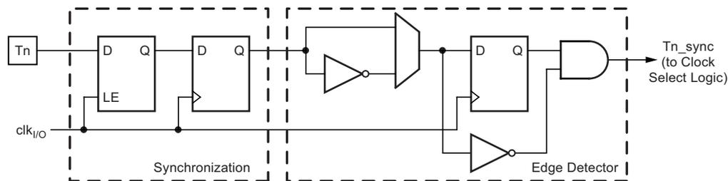
The synchronization and edge detector logic introduces a delay of 2.5 to 3.5 system clock cycles from an edge has been applied to the T1 pin to the counter is updated.
