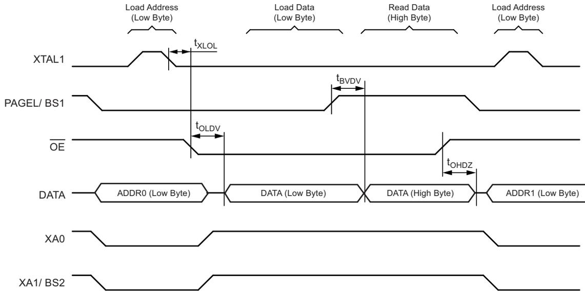
Note: 1. The timing requirements shown in Figure 5-109 (i.e.,  $t_{DVXH}$ ,  $t_{XHXL}$ , and  $t_{XLDX}$ ) also apply to reading operation.
