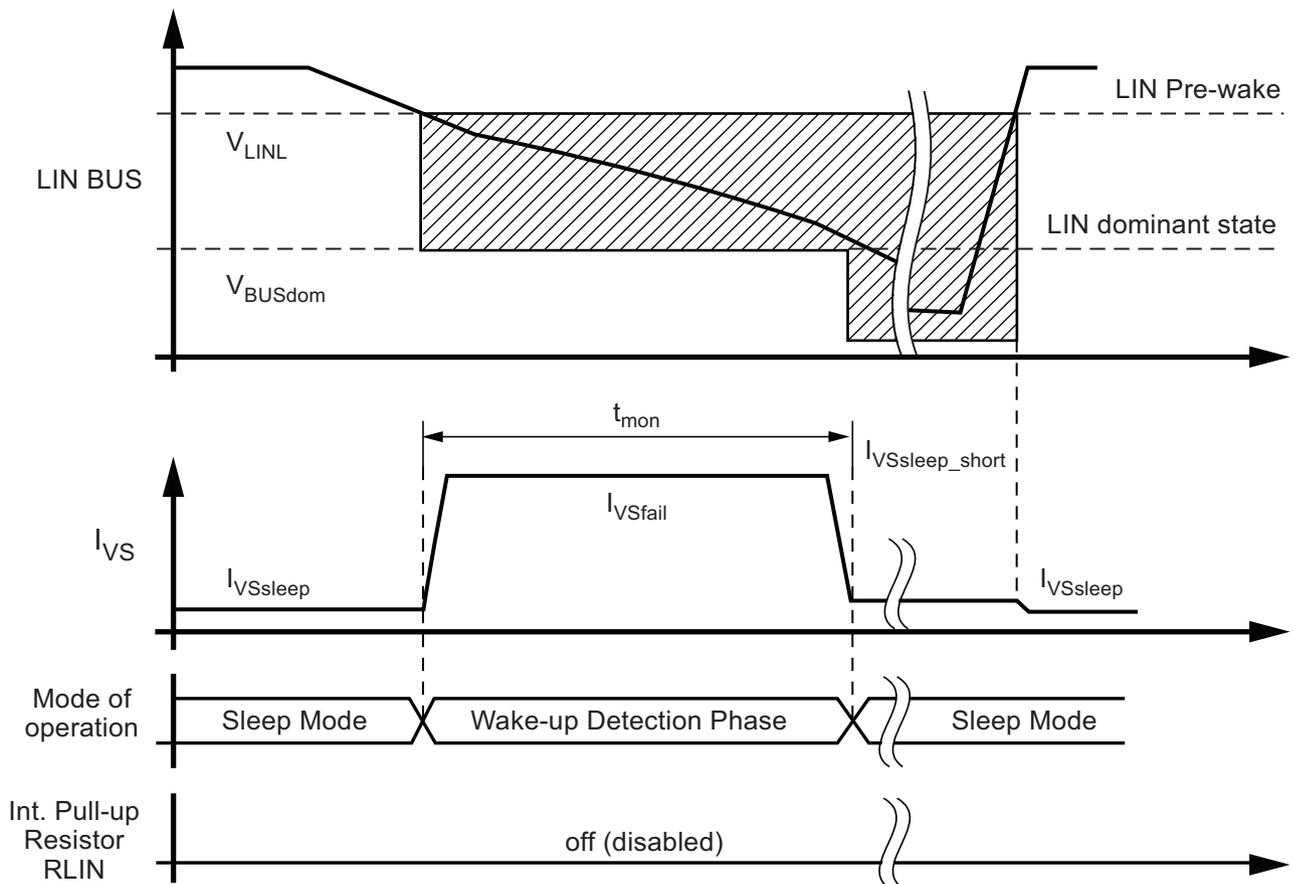
If the LIN-SBC is in Sleep Mode and the voltage level at the LIN bus is in dominant state ( $V_{LIN} < V_{BUSdom}$ ) for a period exceeding  $t_{mon}$  (during a short circuit at LIN, for example), the IC switches back to Sleep Mode. The  $V_S$  current consumption is then  $I_{VSsleep\_short}$  (typ.  $10\mu A$  more than  $I_{VSsleep}$ ). After a positive edge at the LIN pin the IC switches directly to Active Mode.
