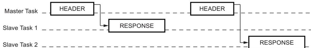
The slave tasks waiting for the data associated with the identifier receives the response and uses the data transported after verifying the checksum.
