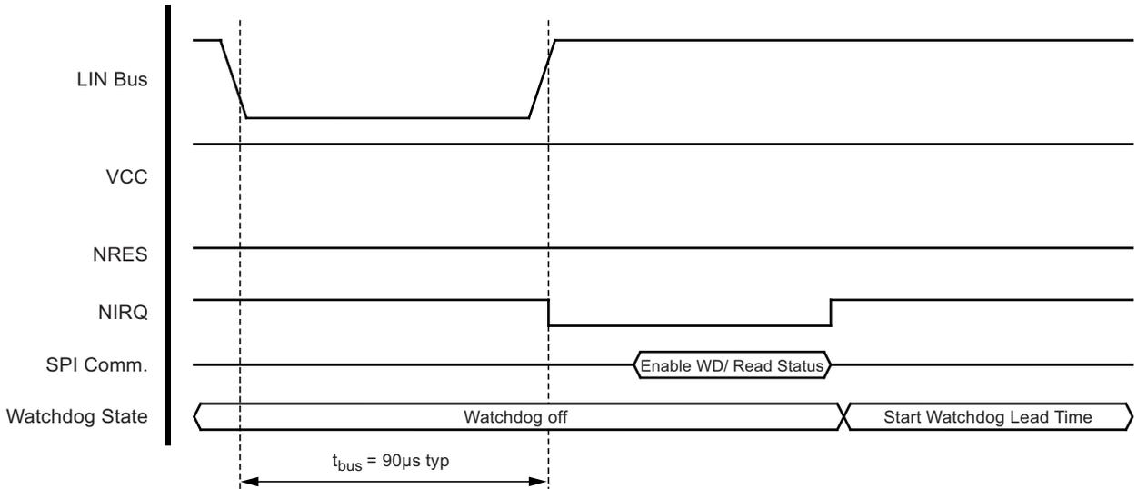
The negative edge on the NIRQ pin indicates a change of conditions, in this case a wake-up request at the LIN bus. The microcontroller can check the IRQ source by assessing the “IRQS1” and “IRQS0” bits in the status register. Note that if a watchdog operation is desired, it must be enabled via the configuration register.
