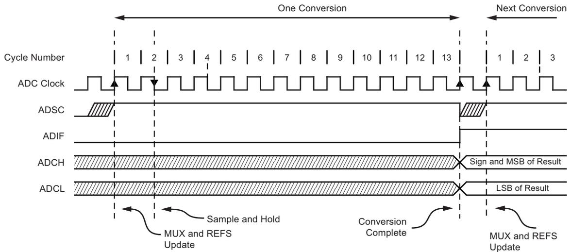
**Figure 5-87. ADC Timing Diagram, Auto Triggered Conversion**
