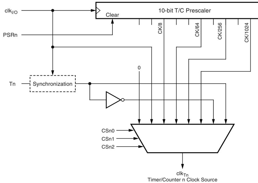
Note: 1. The synchronization logic on the input pin (T1) is shown in [Figure 5-42 on page 134](#).
