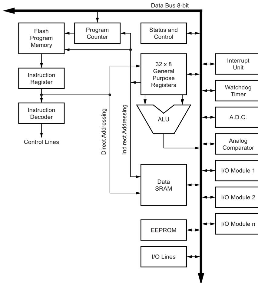
In order to maximize performance and parallelism, the AVR<sup>®</sup> uses a Harvard architecture – with separate memories and buses for program and data. Instructions in the Program memory are executed with a single level pipelining. While one instruction is being executed, the next instruction is pre-fetched from the Program memory. This concept enables instructions to be executed in every clock cycle. The Program memory is In-System Reprogrammable Flash memory.
