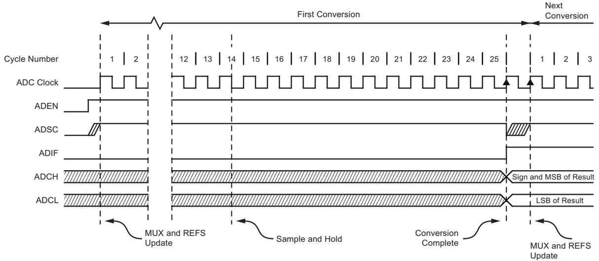
**Figure 5-86. ADC Timing Diagram, Single Conversion**
