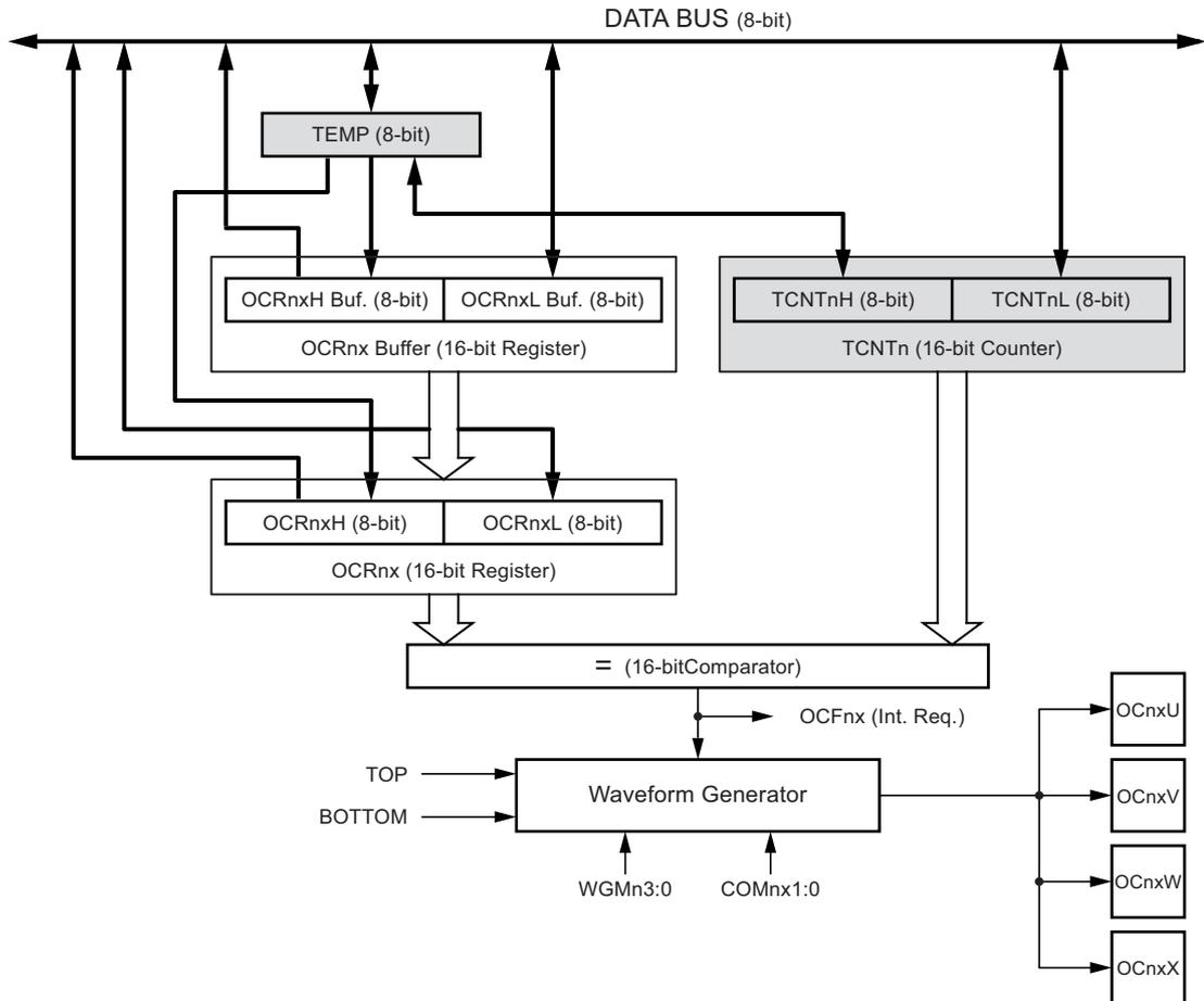
The OCR1A/B Register is double buffered when using any of the twelve Pulse Width Modulation (PWM) modes. For the Normal and Clear Timer on Compare (CTC) modes of operation, the double buffering is disabled. The double buffering synchronizes the update of the OCR1A/B Compare Register to either TOP or BOTTOM of the counting sequence. The synchronization prevents the occurrence of odd-length, non-symmetrical PWM pulses, thereby making the output glitch-free.
