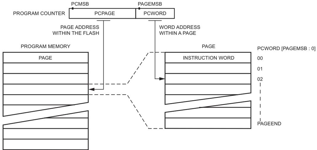
**Figure 5-100. Programming the Flash Waveforms<sup>(1)</sup>**
