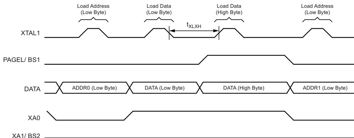
Note: 1. The timing requirements shown in Figure 5-109 (i.e.,  $t_{DVXH}$ ,  $t_{XHL}$ , and  $t_{XLDX}$ ) also apply to loading operation.
