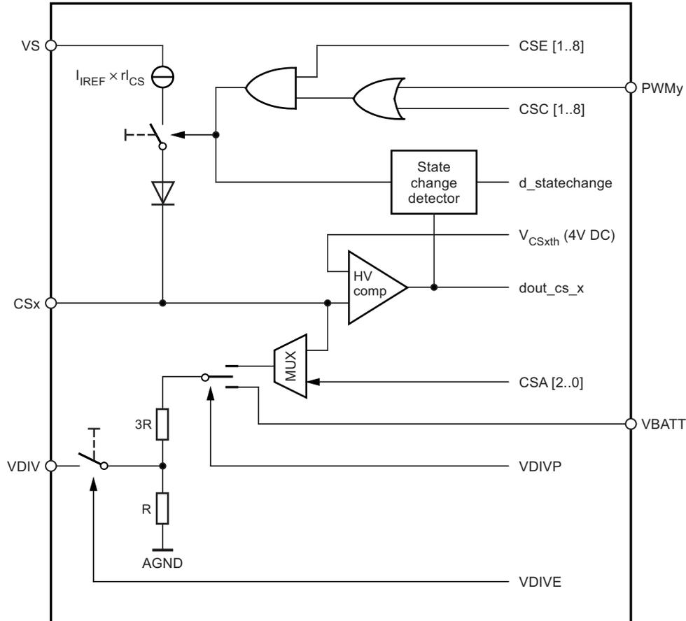
The control signals CSE and CSC are configuration register bits, and unique for each of the eight interfaces. The output signal `dout_cs` of the comparator can be probed via the SPI status register bit `CSxCS`.
