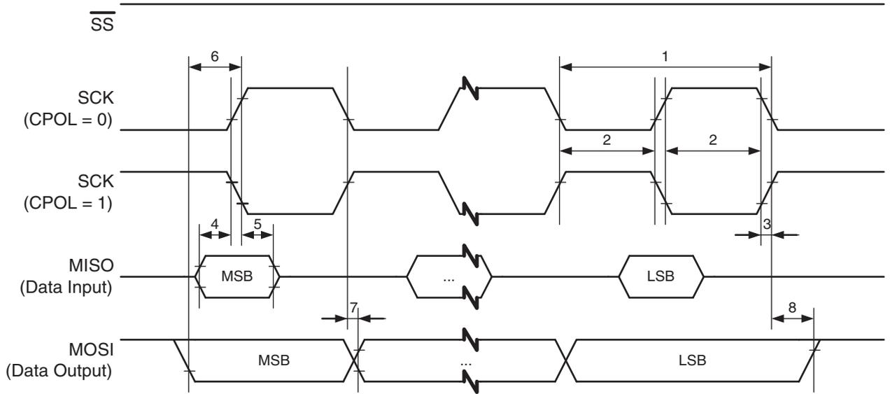
**Figure 5-113. SPI Interface Timing Requirements (Slave Mode)**
