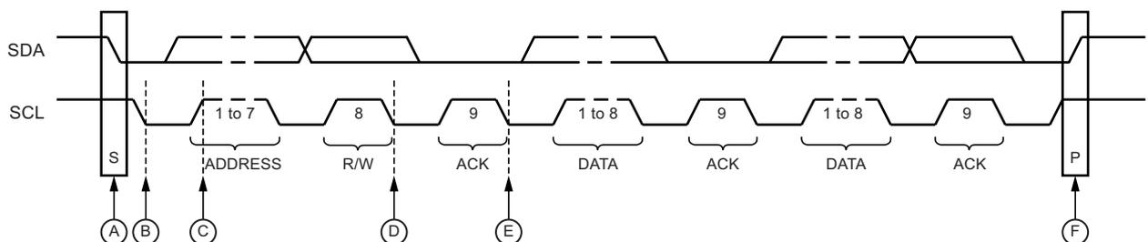
Referring to the timing diagram (Figure 5-66 on page 175), a bus transfer involves the following steps:
