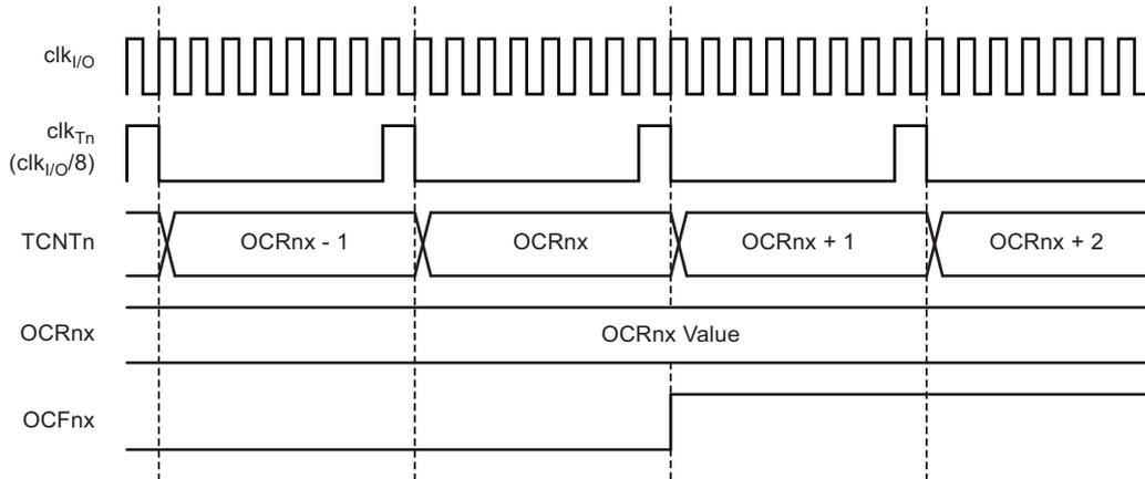
Figure 5-56 shows the count sequence close to TOP in various modes. When using phase and frequency correct PWM mode the OCR1A/B Register is updated at BOTTOM. The timing diagrams will be the same, but TOP should be replaced by BOTTOM, TOP-1 by BOTTOM+1 and so on. The same renaming applies for modes that set the TOV1 flag at BOTTOM.
