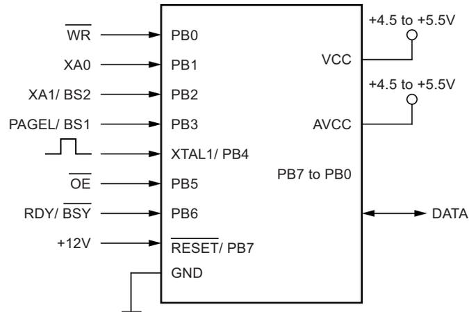
Note:  $V_{cc} - 0.3V < AV_{cc} < V_{cc} + 0.3V$ , however,  $AV_{cc}$  should always be within 4.5 to 5.5V
