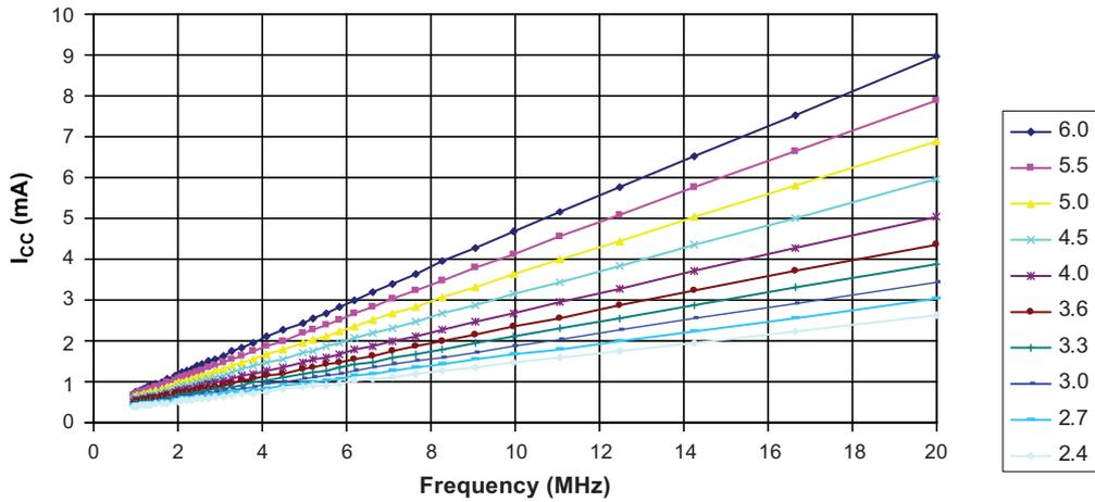
**Figure 5-120. Idle Supply Current versus  $V_{CC}$  (Internal RC Oscillator, 8MHz)**
