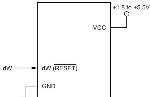
Figure 5-95 shows the schematic of a target MCU, with debugWIRE enabled, and the emulator connector. The system clock is not affected by debugWIRE and will always be the clock source selected by the CKSEL Fuses.
