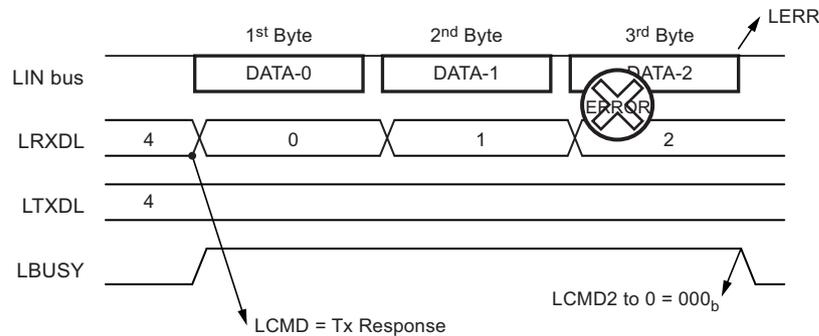
Note: Information on response (ex: error on byte) is only available at the end of the serialization/de-serialization of the byte.
