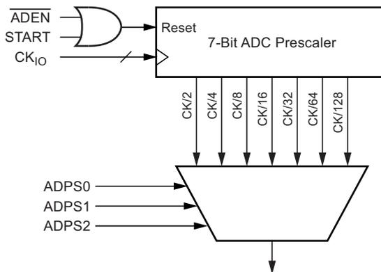
By default, the successive approximation circuitry requires an input clock frequency between 50kHz and 200kHz to get maximum resolution. If a lower resolution than 10bits is needed, the input clock frequency to the ADC can be higher than 200kHz to get a higher sample rate.
