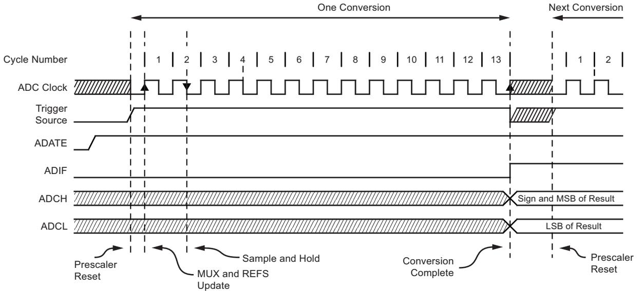
**Figure 5-88. ADC Timing Diagram, Free Running Conversion**
