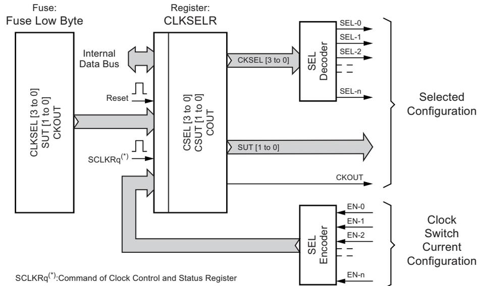
The CLKSELR register contains the CSEL, CSUT and COUT values which will be used by the 'Enable/Disable Clock Source', 'Request for Clock Availability' or 'Clock Source Switching' commands.
