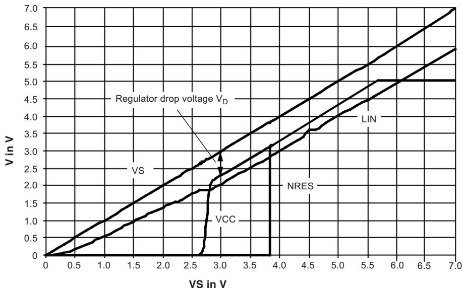
Please note that upper graph is only valid if the VS ramp-up time is much slower than the VCC ramp-up time  $t_{VCC}$  and the NRES delay time  $t_{reset}$ .
