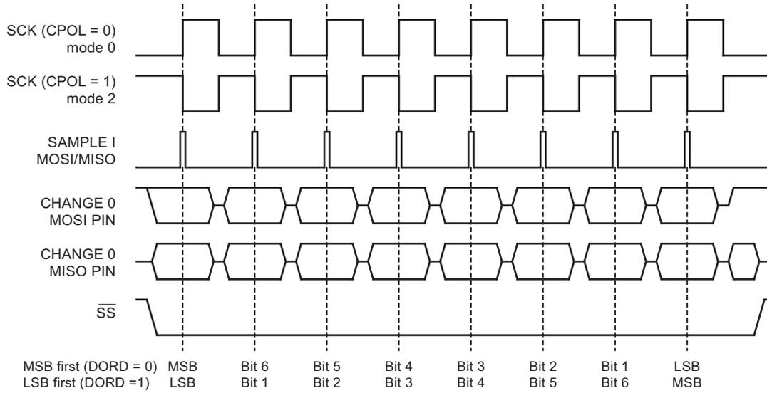
**Figure 5-61. SPI Transfer Format with CPHA = 1**
