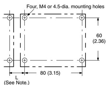
Note: If more than one Power Supply is installed in a row, keep a distance of 20 mm min. (L = 20 mm min.) between each adjacent Power Supply.
