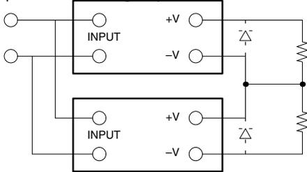
When connecting the Power Supplies in series with an operation amplifier, connect diodes to the output terminals as shown by the dotted lines in the figure. No diodes are required with S82K 90-/100-/240-W models.
