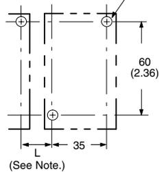
Note: If more than one Power Supply is installed in a row, keep a distance of 20 mm min. (L = 20 mm min.) between each adjacent Power Supply.
