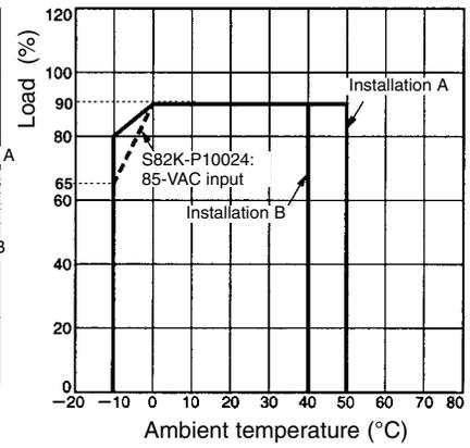
Note: When using the 7.5-W single-output models within the input voltage range between 90 and 110 VDC, the load rate will become 90% or less.
