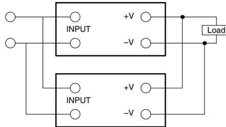
Note: When operating the S82K-P10024 or 240-W model in parallel operation, set the switch to "PARALLEL." Refer to the derating curve for the rated current under this operation.
