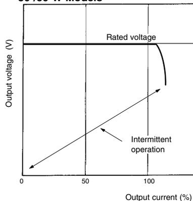
Note: Do not short-circuit the output terminals of the S82K or use the S82K with excessive output current for a long time, otherwise the internal circuitry of the S82K may be deteriorated or damaged.
