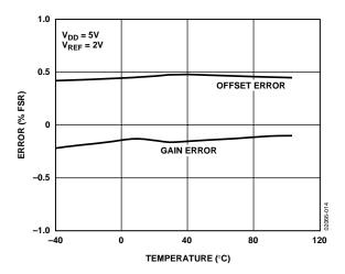
Figure 14. AD5306 Offset Error and Gain Error vs. Temperature
