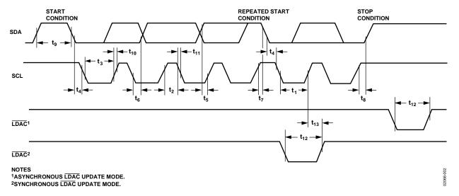
Figure 2. 2-Wire Serial Interface Timing Diagram
