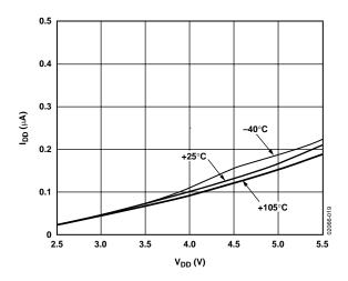
Figure 19. Power-Down Current vs. Supply Voltage
