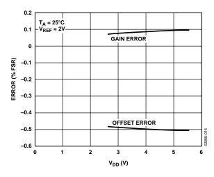
Figure 15. Offset Error and Gain Error vs. V<sub>DD</sub>
