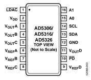
Figure 3. Pin Configuration
