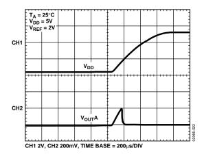
Figure 22. Power-On Reset to 0 V
