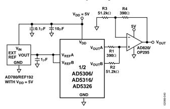
Figure 40. Coarse/Fine Adjustment
