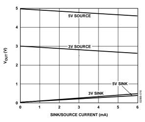
Figure 16. V<sub>OUT</sub> vs. Source and Sink Current Capability
