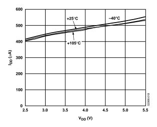
Figure 18. Supply Current vs. Supply Voltage
