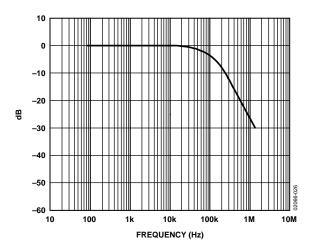
Figure 26. Multiplying Bandwidth (Small-Signal Frequency Response)
