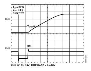
Figure 21. Half-Scale Settling (1/4 to 3/4 Scale Code Change)
