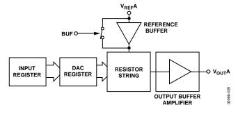
Figure 29. Single DAC Channel Architecture
