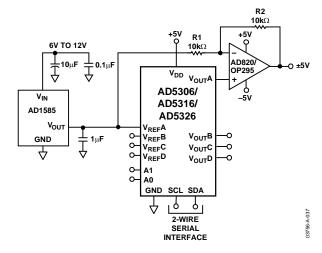
Figure 37. Bipolar Operation with the AD5306/AD5316/AD5326
