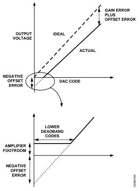
Figure 4. Transfer Function with Negative Offset
