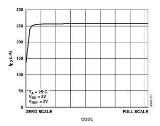
Figure 17. Supply Current vs. DAC Code
