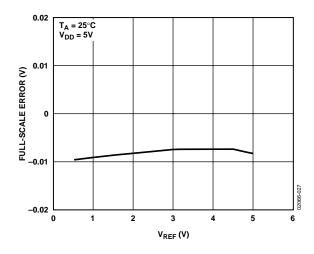
Figure 27. Full-Scale Error vs. VREF
