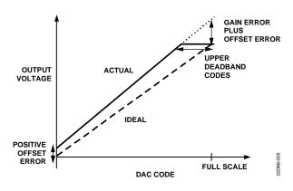
Figure 5. Transfer Function with Positive Offset ( $V_{REF} = V_{DD}$ )
